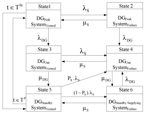
Fig. 1. Six-state model of DG operated in peak shaving and standby
